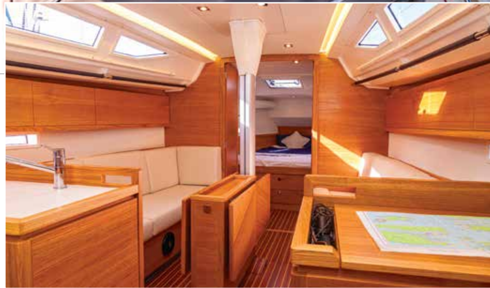
Interior joinery is in light oak and all made at the yard. Drawers are in wood throughout and frames and fiddles are solid. The double-width door to the forecabin creates a feeling of space
