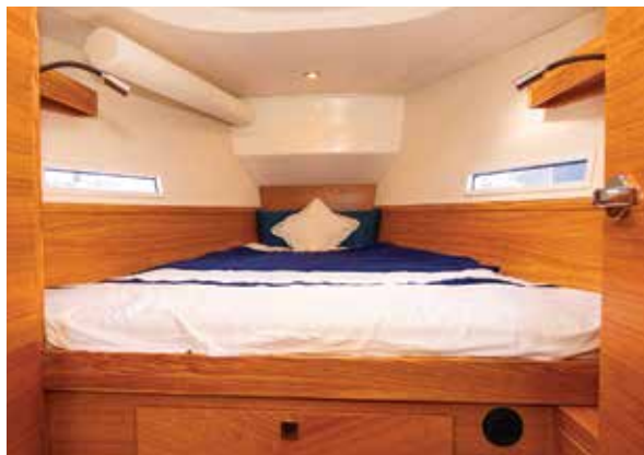
The optional bowsprit for an asymmetric spinnaker retracts into a tube in the forecabin. A second water tank can fit beneath the berth
