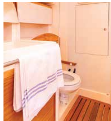
The most popular layout has the heads aft and a door opening into a wet locker
