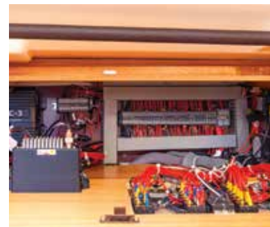
Electrics are neatly laid out behind a hinge-down panel above the chart table
