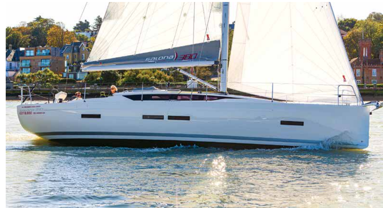
BELOW: The flying bow, with the knuckle clear of the water, becomes immersed to lengthen the waterline under way
