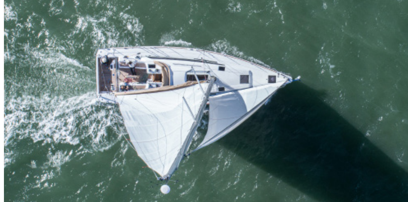
ABOVE The J&J designed hull lines are conservative with modest beam and some taper aft
